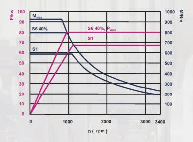
Spindle 125 mm (4.9"), 2,500 rpm as main spindle or as sub spindle for all machines of the series TS-TTS
