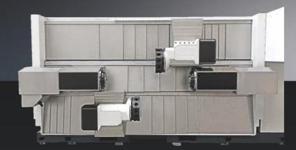
In addition, flexibly utilizable steady-rests are possible, each optionally movable in two CNC axes on a cross-slide, in order to be brought quickly and precisely from a protected park position to the usage position.
