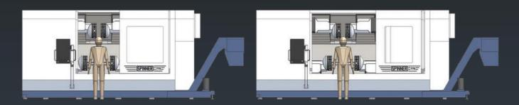
There is also a choice of two bed lengths with normal and extended Z-stroke.
