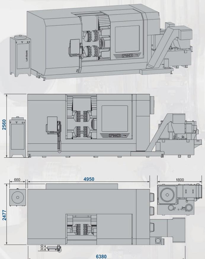
Shown with optional coolant system 80 bar and coolant temperature control Further variants on request
