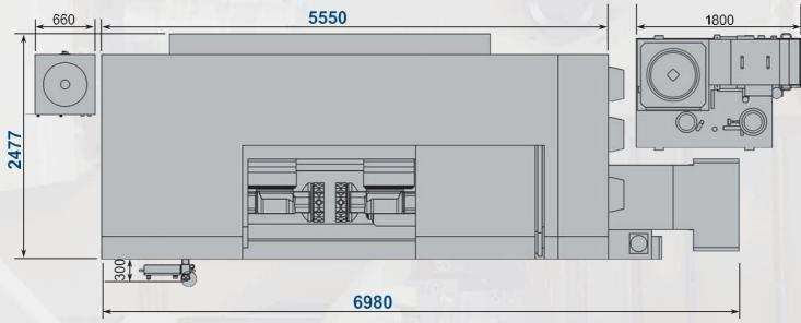
Shown with optional coolant system 80 bar and coolant temperature control Further variants on request
